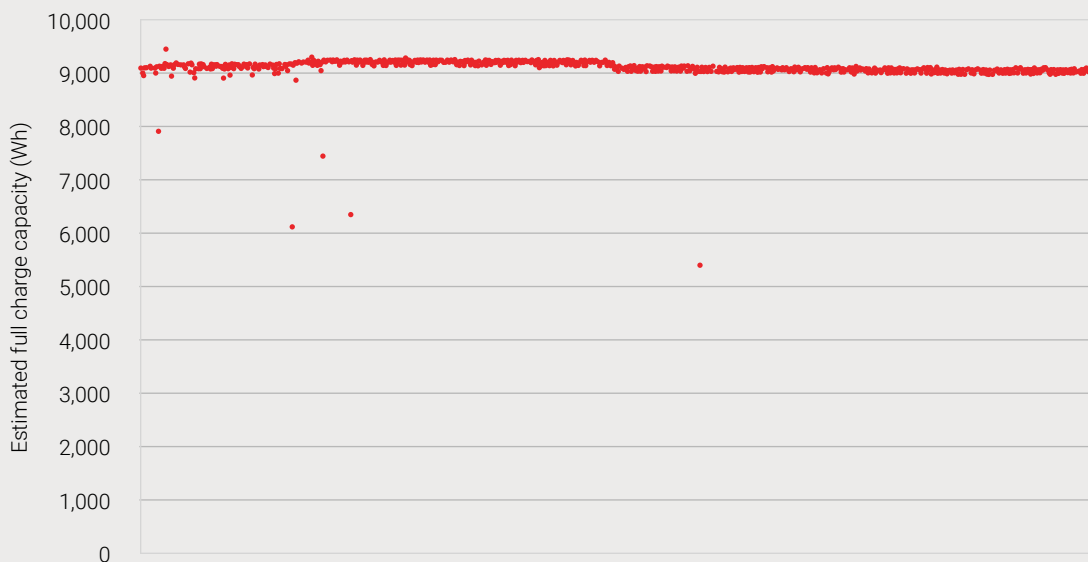
Figure 9: Estimated full charge capacity per cycle by the BYD HVM battery pack
