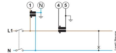
**4c 2 PHASES, 3 WIRES - CT (Step: 4c)**
