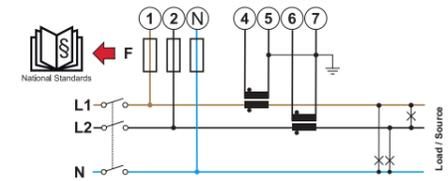
**4d 2 PHASES, 3 WIRES - VT/CT (Step: 4d)**
