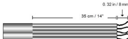
Figure 28: Insulation stripping – AC
