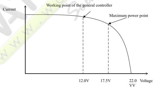
As a charging stage, MPPT can't be used alone. It must be combined with ascending charge, floating charge, equalizing charge to complete the battery charge.
