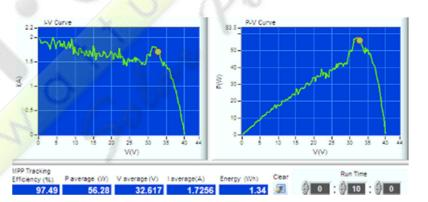
4 There's wide-range shadow covered PV module, the tracing efficiency is 99.64%.
