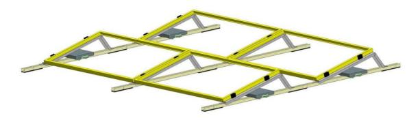
Place the panels on the mounting triangles and clamp them with the appropriate end and centre clamps.
