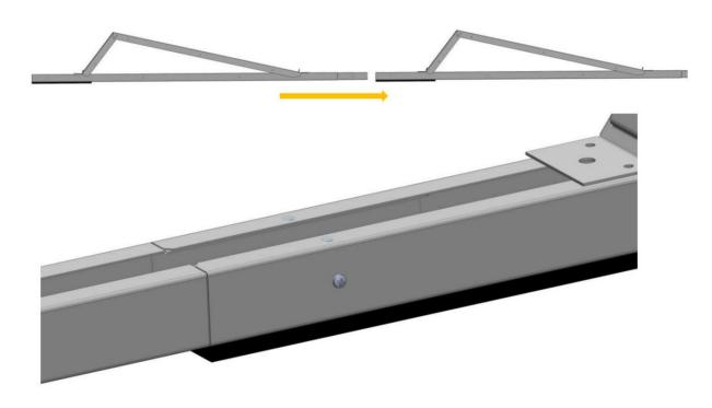
STEP 2: Attach the end rubber to the end of the column
