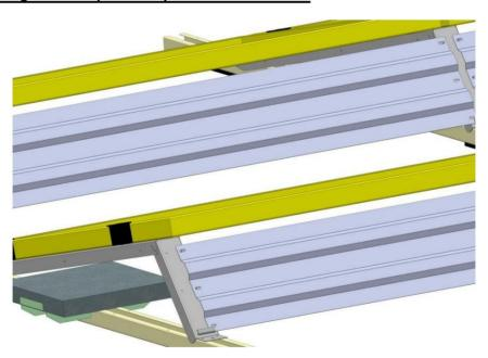
Place the SolarSpeed backplate on the back of the SolarSpeed mounting triangle and fasten using stainless steel sheet metal screws (Ø6.3) (minimum 4 per backplate).
