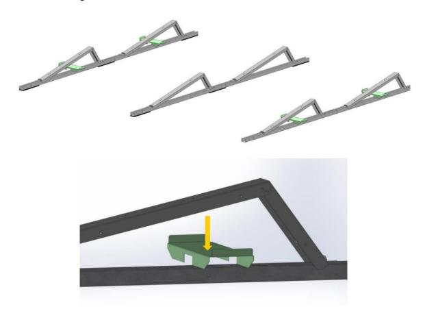
After mounting the SolarSpeed backplate (step 6), it is also possible to place additional ballast on the end of the setup/columns.
