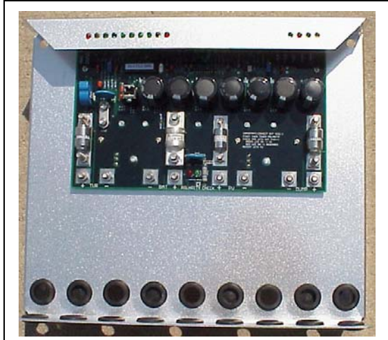
Figure 14: PowerCenter with Cover Removed
