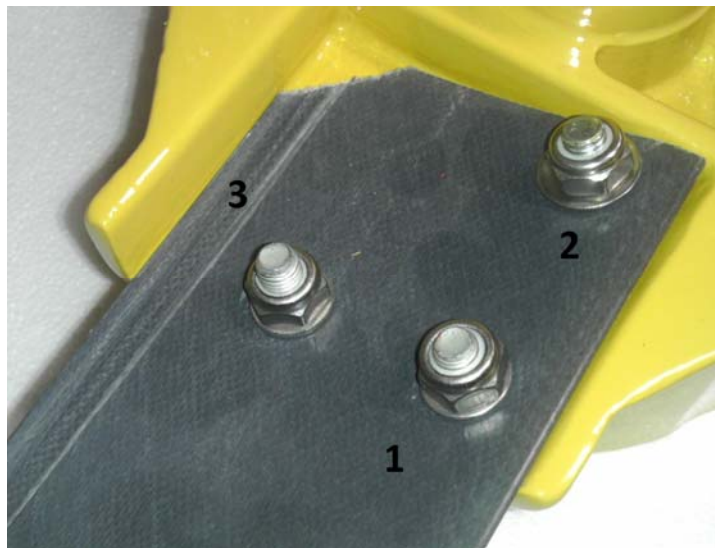
Figure 10: Nut Tightening Order
