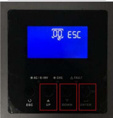
**Note:** Axpert Inverter can only be waked up via battery, if the battery is turned off due to over-discharge, over temp. or other reasons, in order to wake up the inverter you need turn on the battery manually.
