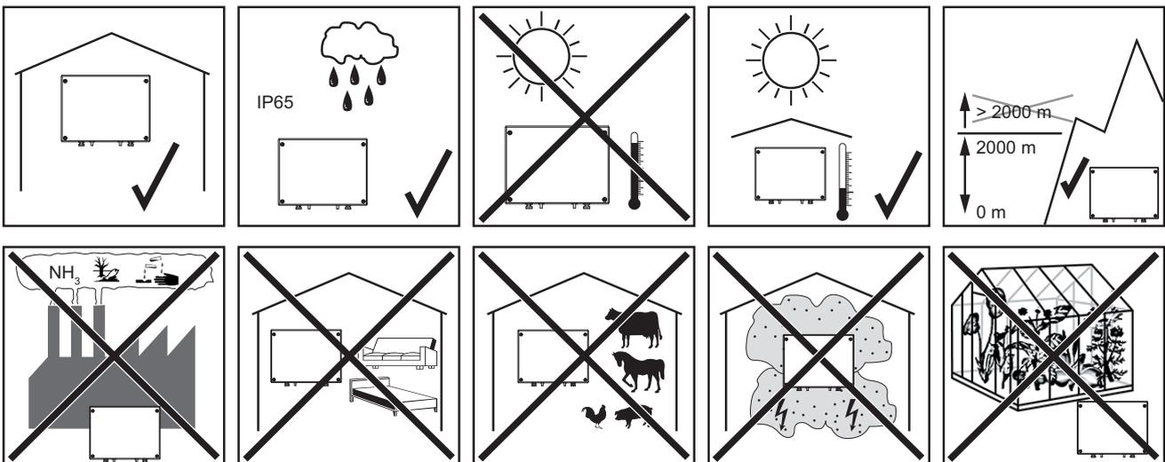
Possible assembly positions when using outdoors:
